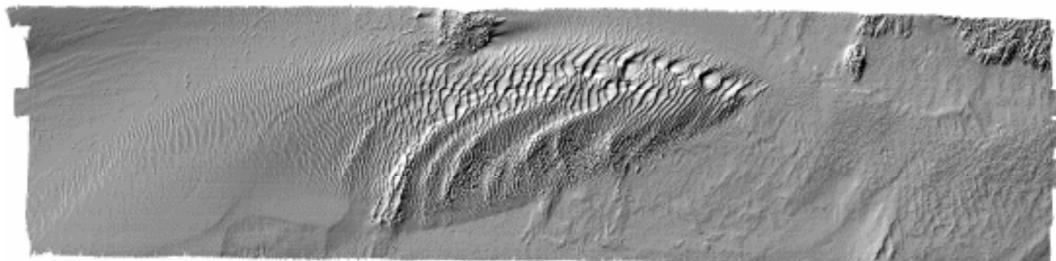
**Fig.8 Seabed DTM reconstructed by signal blend technique**
