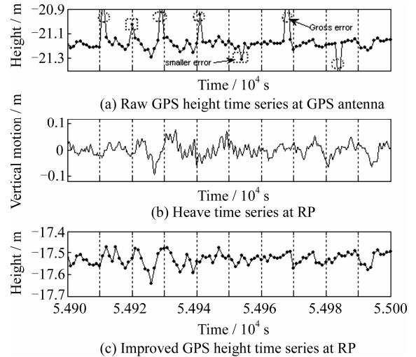
Fig.1 Heave modification and the relation between heave series and GPS series
