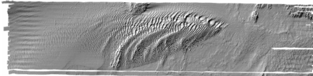
Fig.5 Seabed DTM constructed by traditional multibeam data processing method
